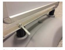
Attach frame to springs and base: align the poster frame to the springs and attach them by tightening together with the smaller bolts and spanner.
