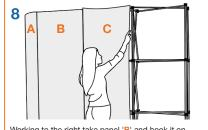
Working to the right take panel 'B' and hook it on to the yellow nodes at the top so it butts up against panel A on the left and takes up the other half of the magnetic bar. Work across to the right adding panels until you get to the opposite D-end panel which will wrap around to the rear as before.
