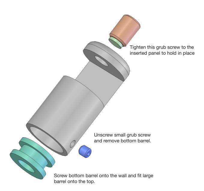
Tighten small grub screw once in place to secure.
